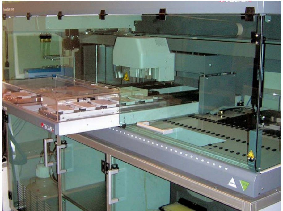
Figure 2: The Freedom EVO system to produce and normalize the genome-wide esiRNA libraries. For UV measurements to determine the RNA concentration, the RoMa arm lifts the plates down from the work table to the GENios Plus reader, which is placed on the level below, as seen in the lower right corner.
