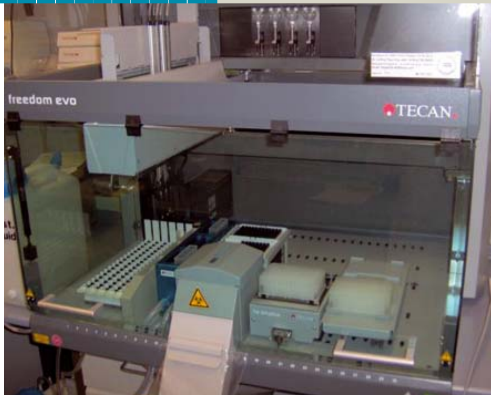
Configuration of the Freedom EVO workstation used, including sample trays, washing station, chilled reagent trough holder, tip holder, tip dropping station and horizontal shaker with deep-well plate
