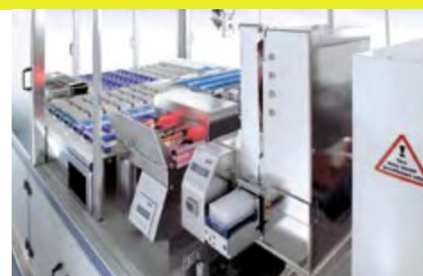
Dosage and Solution Preparation Station with tube sealing and capping.
