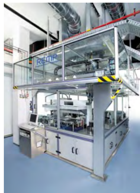
The REMP Dosage and Solution Preparation station.
