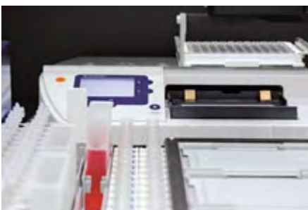
Transportation of amaxa’s Nucleocuvette™ plate to the 96well Shuttle.
