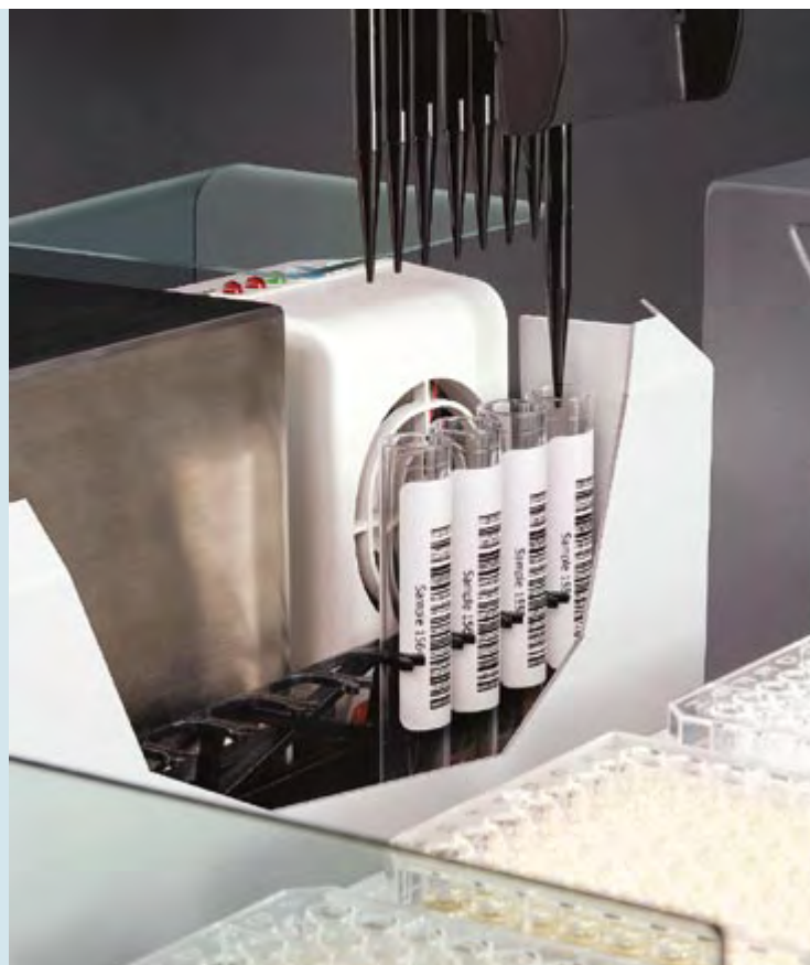
Close-up view of the Te-PoolSafe balance dispensing sera into the pooling tube
