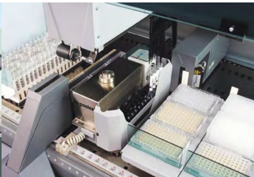
Dispensing into the pooling tube on the Te-PoolSafe balance
