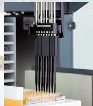
Capabilities of the 8 Plus 1 Access arm; eight-tip pipetting and one tip independent action
