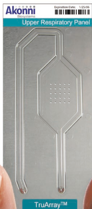
Akonni's TruArray™ microfluidic device
