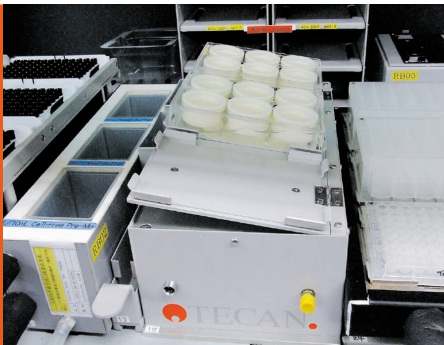
(Below) The Protein Research Group's Freedom EVO workstation set-up, including the custom-made tilting carrier which is tilted to the right (as shown) when reaction solutions are collected from flat-bottom wells
