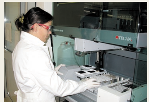
Figure 1: Comparison of the automated (left) and the conventional CTAB-based protocol (right) for plant DNA extraction (Step 2). The automated protocol uses the Wizard® Magnetic 96 DNA Plant System (Promega) on a Tecan Freedom EVO 100 workstation with four pipetting channels and the Te-MagS magnetic separation unit. The manual procedure for the preparation of plant lysate from 48 samples (Step 1) remains identical for both extraction types. Fully automated steps are coded in green, while those requiring manual intervention are coded in red.
