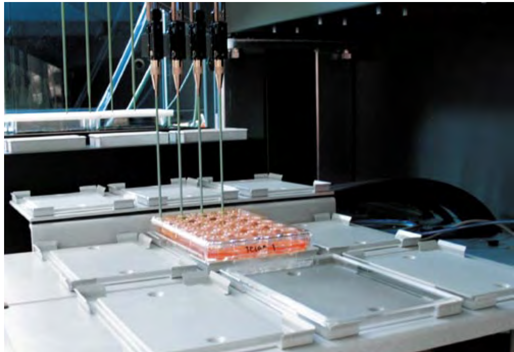
Fixed tips on the liquid handling arm add media to cultured cells in the Millicell ® -24 filter plate
