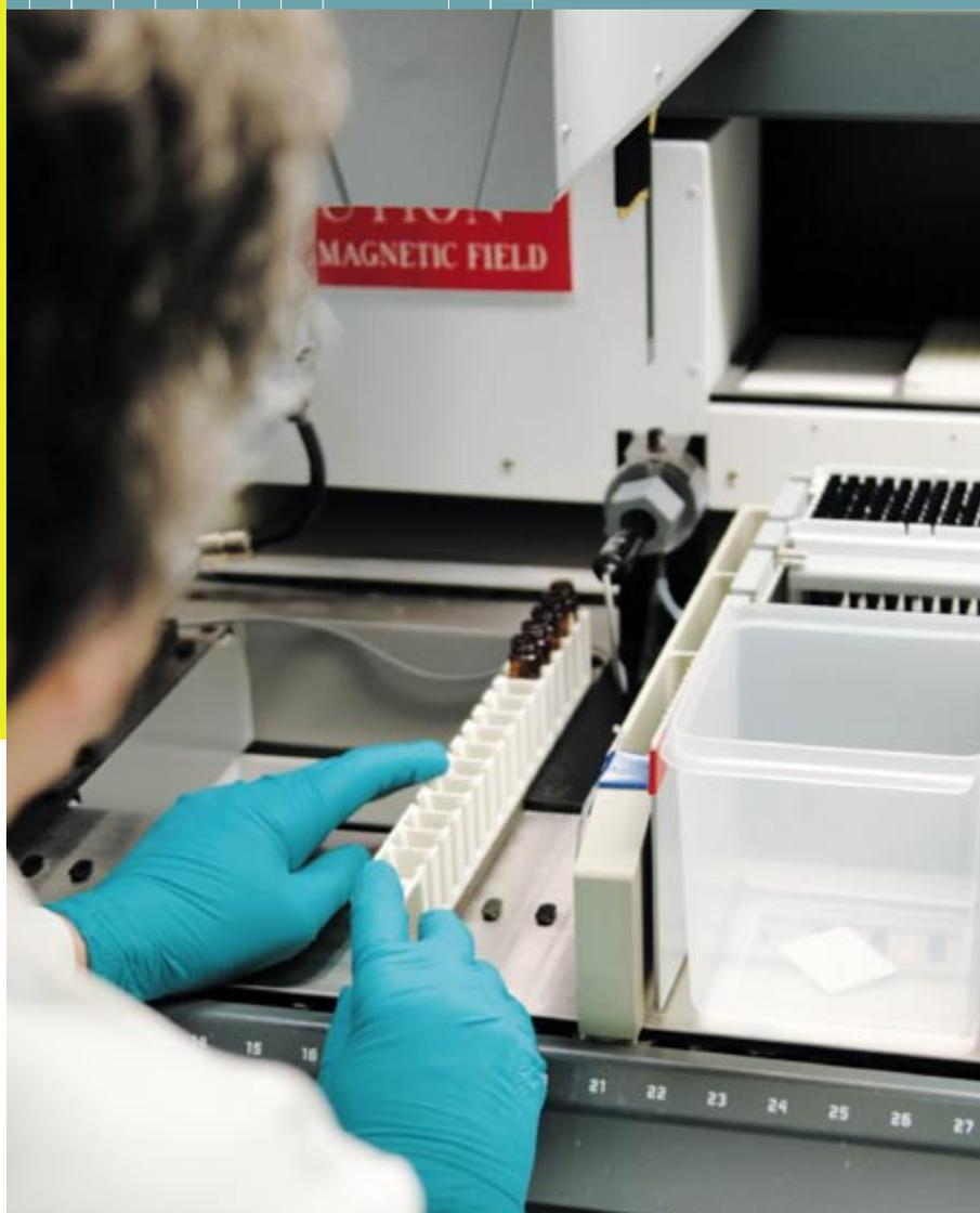
*Rod Kittlety loads the carrier which holds the pH calibration buffers*
