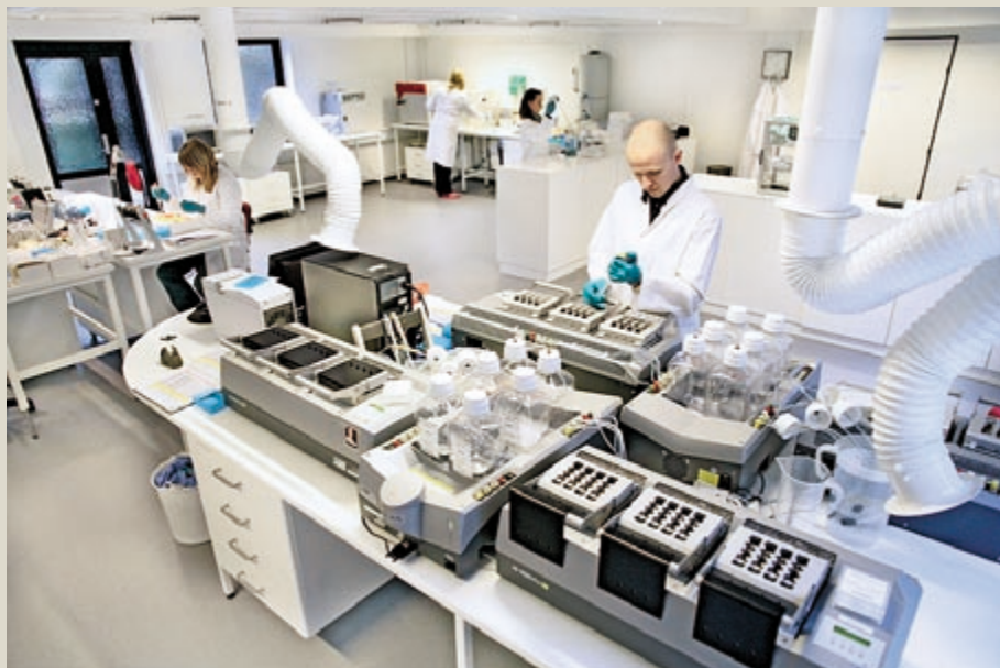
Loading samples into the HS 4800 Pro hybridization station in the service department at Exiqon
