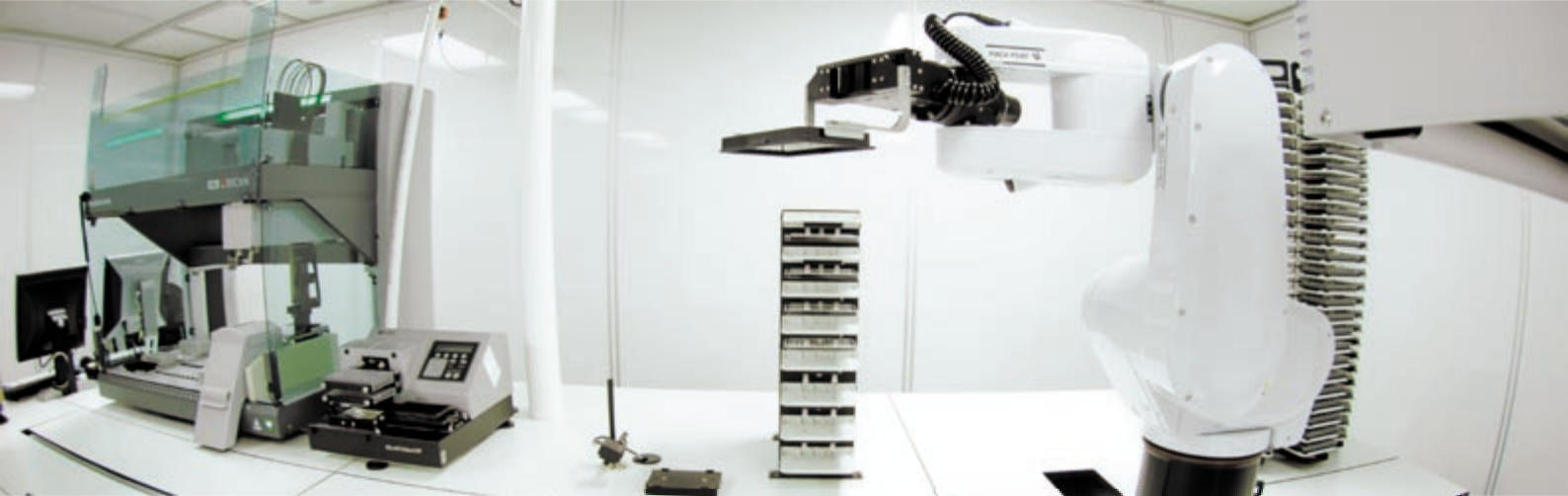
The Freedom EVO 100 has been integrated with a microplate heat sealer and is accessed by a robotic arm
