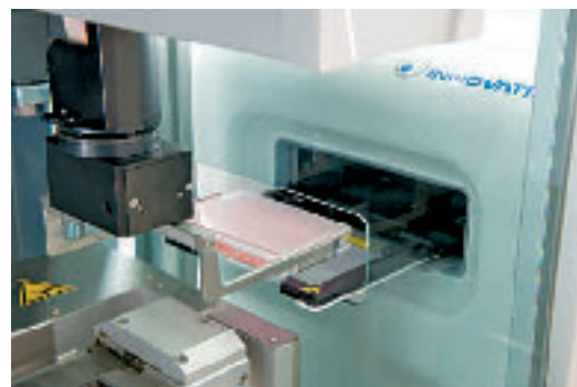
The Freedom EVO workstation, combined with innovatis' Cellavista automated image-based platform technology, allows full automation of a wide range of cell-related processes.
