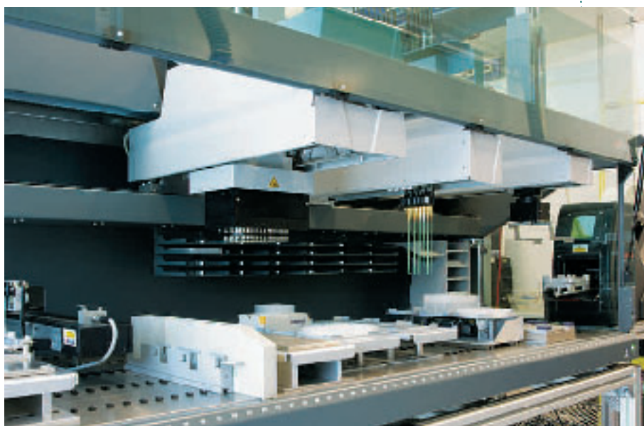
The Freedom EVO platform in Compound Management and Analysis prepares compound plates for screening.
