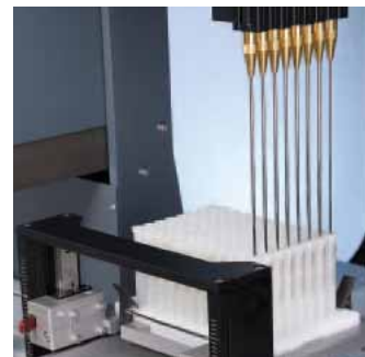
Column flow is controlled via pressure-tight inlets
