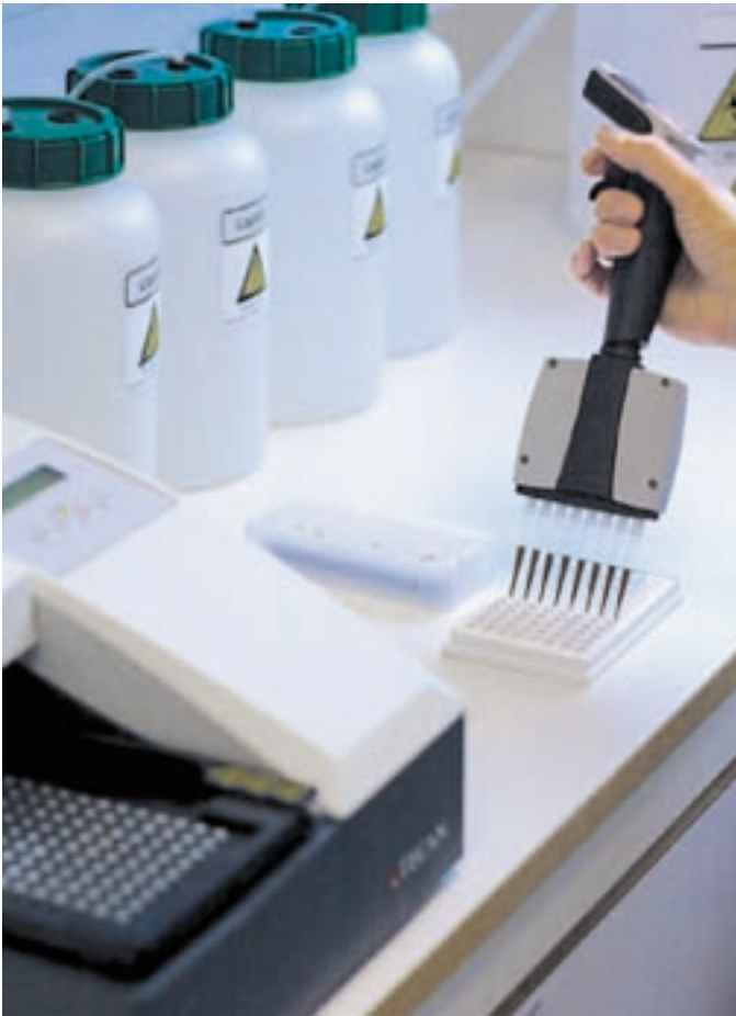
HydroFlex with smart-2 MBS magnetic carrier for bead washing
