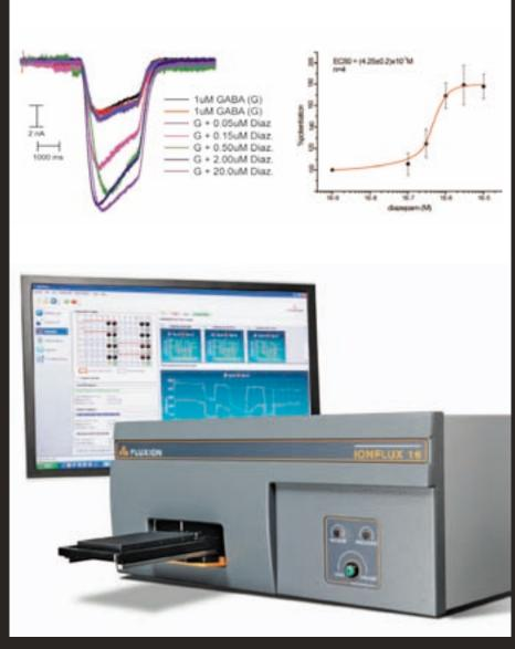
**IonFlux system for high throughput electrophysiology.** The IonFlux system is designed to operate much like a plate reader. Plates are preloaded with cells, compounds, and reagents using the Freedom EVO platform. Once filled, plates are fed automatically into the instrument. All fluidic control necessary to trap cells and deliver compounds is handled within the instrument and integrated electrodes record ion channel currents.
