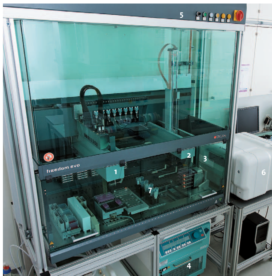
1. LiHa Arm with four standard tips and four wide bore tips for cell pipetting 2. Robotic Manipulator (RoMa) Arm equipped with eccentric gripper fingers 3. Flipper module with four positions for RoboFlasks 4. Centrifuge Rotanta 46 RSC Robotic (Hettich, Germany), mounted under the worktable 5. Clean air hood 6. Cellavista System 7. Orbital shakers Not shown: Optional incubator for fully automated system (37 °C, 5 % CO 2 , humidified atmosphere)
