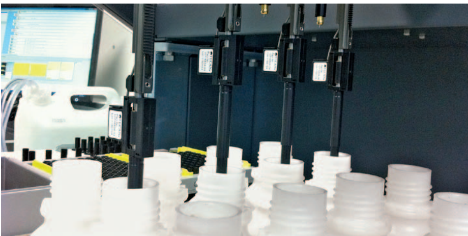
Aliquoting urine samples from 200 ml bottles using the LiHa Arm with 5 ml disposable tips
