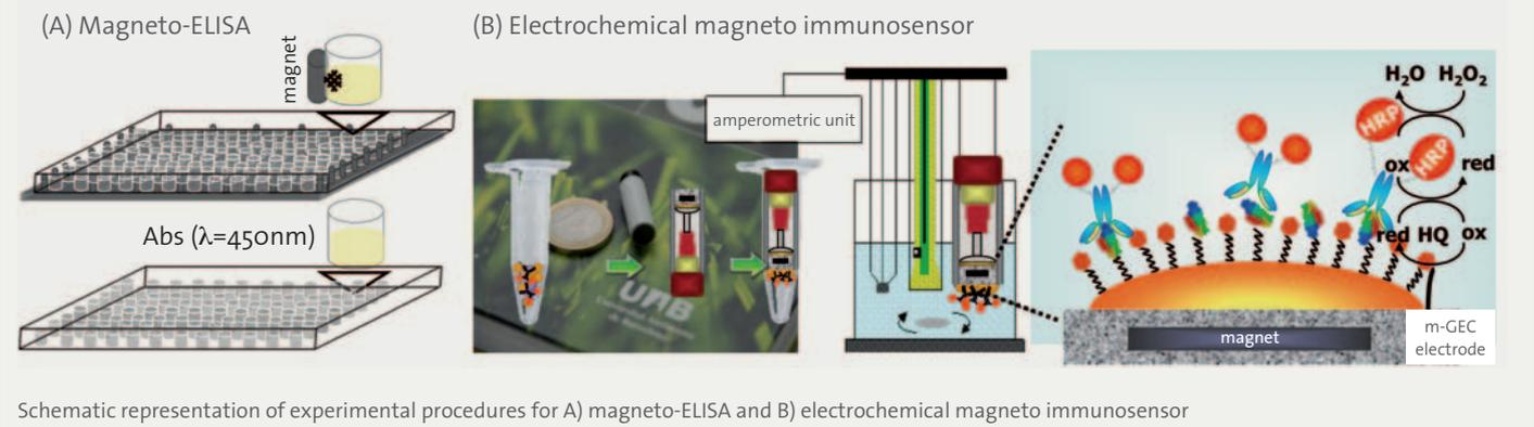
Schematic representation of experimental procedures for A) magneto-ELISA and B) electrochemical magneto immunosensor
