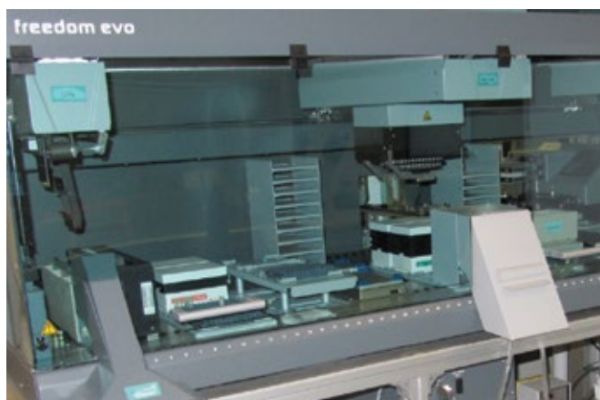
Freedom EVO 200 with eight-channel Liquid Handling Arm, MCA 96 and integrated gripper, carousel and incubator (StoreX 110, LiCONic)
