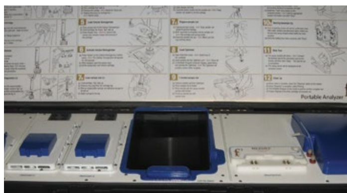
F Cubed's NESDEP analyzer enables single-stranded DNA to be detected in a microfluidic setting
