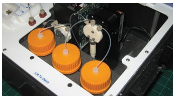
The Cavro Smart Valve and Cavro Centris Pump are key components of the NESDEP analyzer
