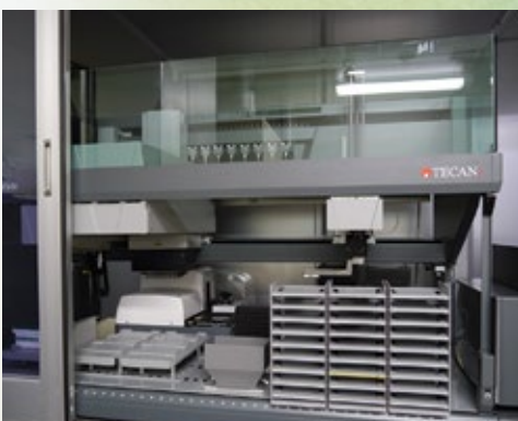
The department's Freedom EVO workstation has a fully integrated HydroSpeed plate washer and Infinite F200 PRO microplate reader
