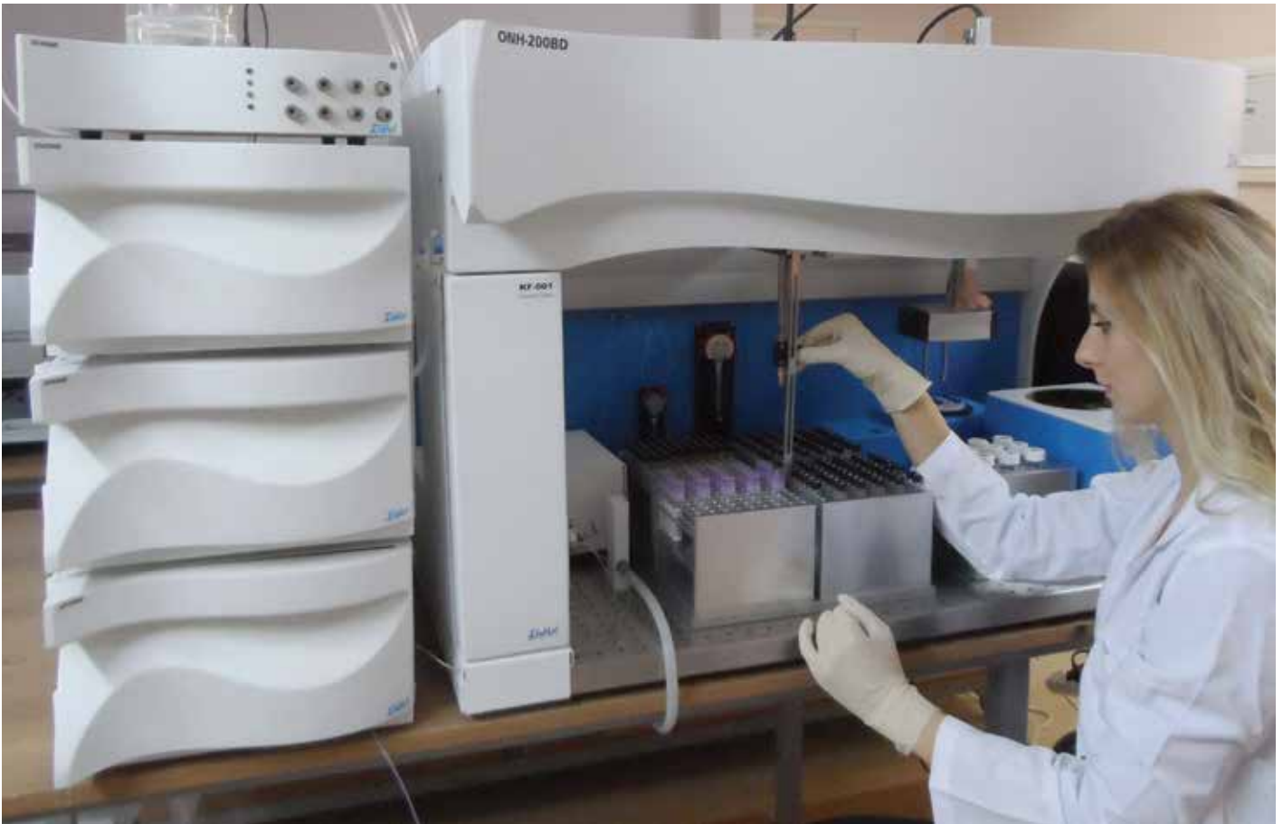
Kübra Balyemez shows how the Cavro Omni Robot has been incorporated into Zivak's 25-OH Vitamin D 2 -D 3 HPLC Analyzer
