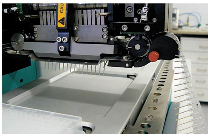
The mosquito provides positive displacement pipetting down to 25  $\text{nl}$
