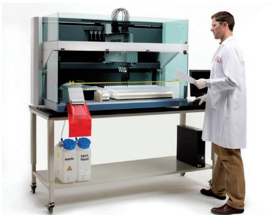
The Procleix SP combines blood pooling and archiving on a single instrument
