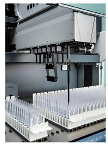
The instrument's 8-channel Liquid Handling Arm offers efficient throughput
