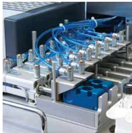
The custom bioreactor block can be accessed by the system’s LiHa Arm
