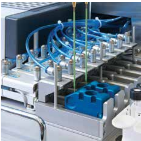
The custom bioreactor block can be accessed by the system’s LiHa Arm
