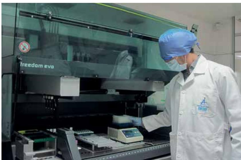
The Freedom EVO offers walkaway automation of nucleic acid extraction and real-time PCR protocols
