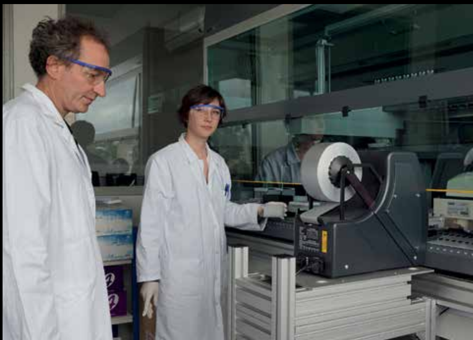
The laboratory's Freedom EVO platform has a range of integrated devices to offer almost complete automation of its workflow
