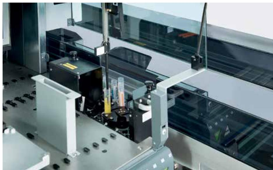
The LiHa Arm can pipette samples directly from tubes on the sample track
