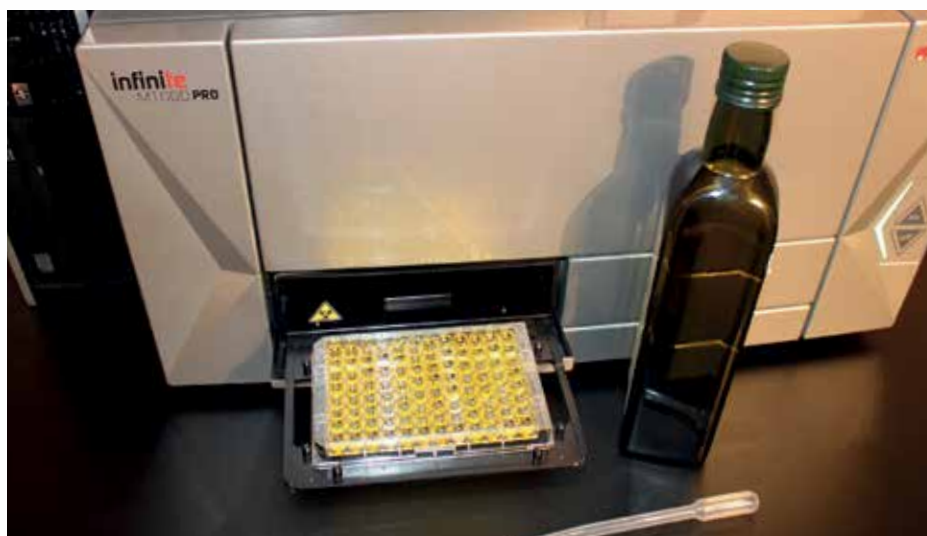
Surveillant’s label-free technique relies on the Infinite M1000 PRO’s ability to create consistent fluorescence spectra
