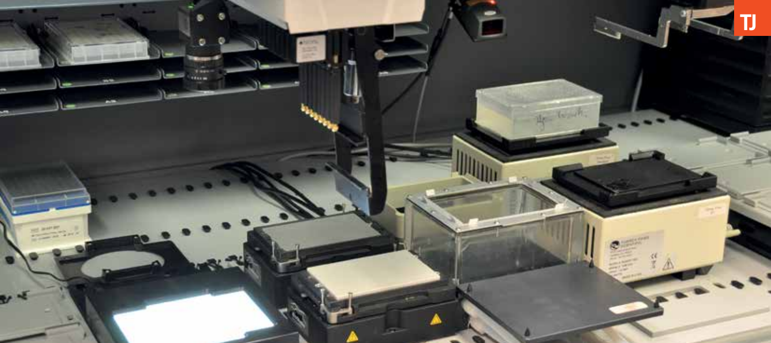
Integration of the Pickolo and other third-party devices onto the workstation proved key to automating the DNA assembly workflow
