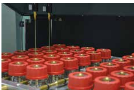
The LiHa Arm's fixed tips allow direct transfer of samples from fermentation flasks...
