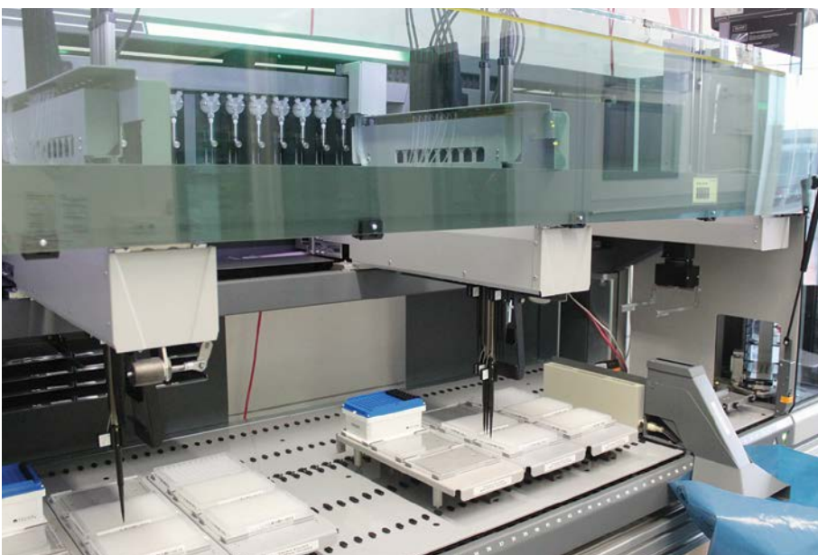
Automation on a Freedom EVO platform enables cost-effective, high throughput HLA typing
