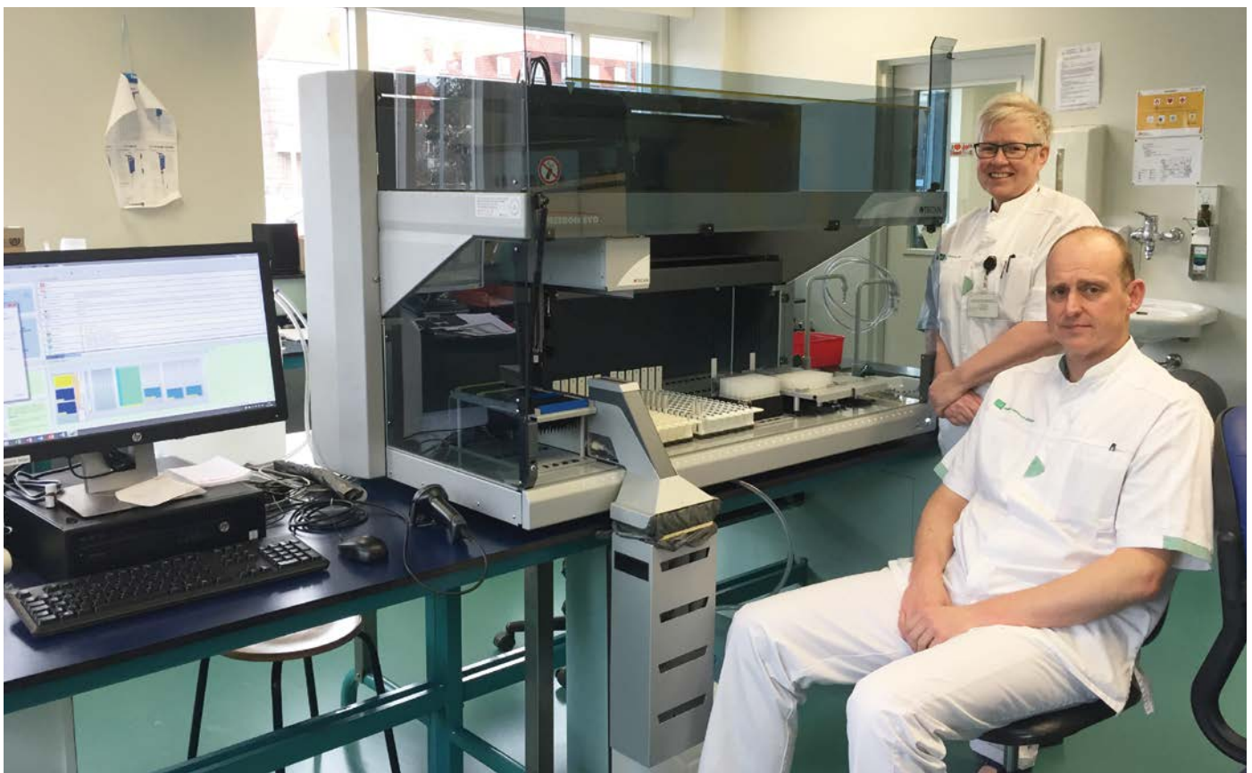
NWZ's Freedom EVO offers fully automated pre-analytical processing
