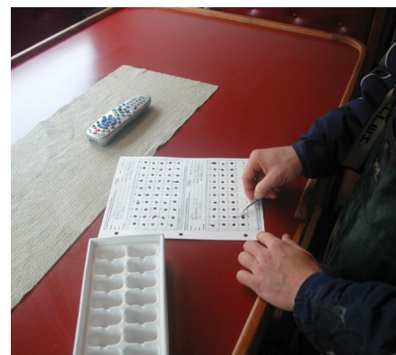
Samples are mounted on filter paper and sent to the laboratory
