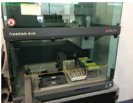
The Freedom EVO streamlines post-analytical sample preparation, simplifying the biobanking workflow
