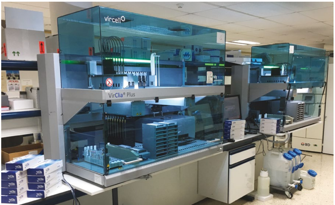
The Freedom EVO-based VirClia Plus system offers walkaway processing of 96 samples in three hours
