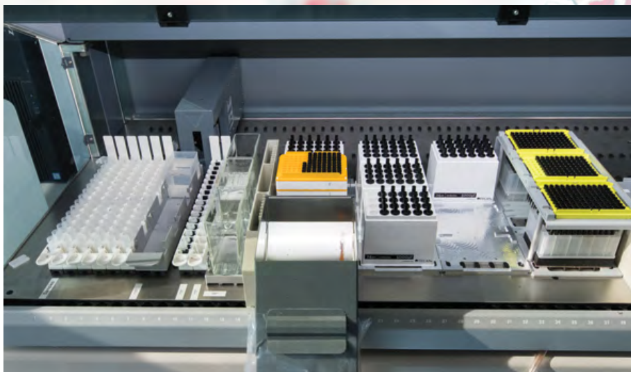
Epigenomics' automated workflow requires integration of various labware formats and ancillary devices onto the workdeck
