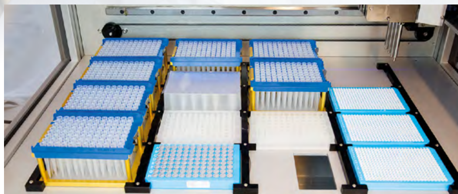
The AusDiagnostics Ultra-Plex 96 uses four Cavro ADPs to conduct a two-step PCR workflow in as little as 3.5 hours
