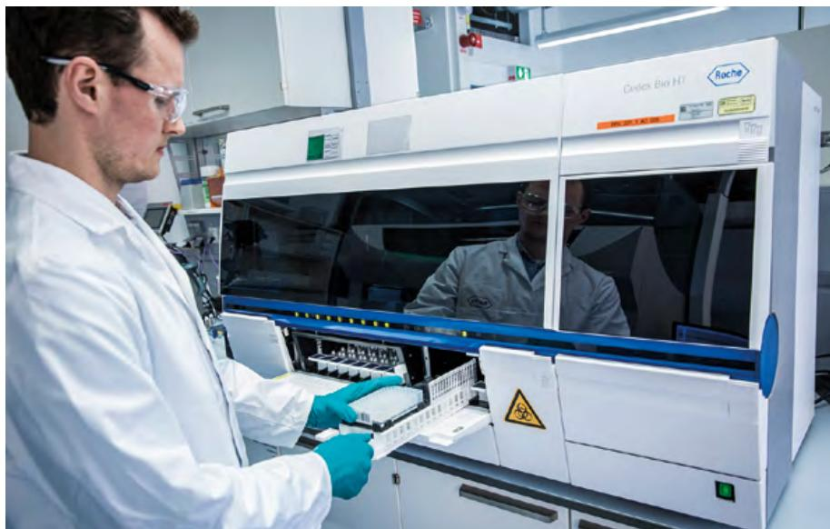
The Cedex Bio HT Analyzer's microplate-based sampling system allows easy transfer of samples between devices
