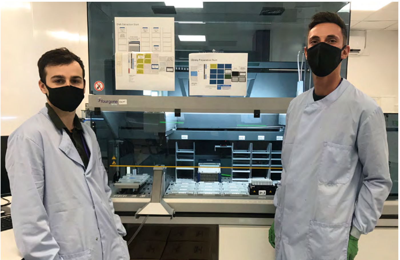
The Yourgene SP150 is based on Tecan’s Freedom EVO platform
