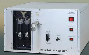
The Cavro Centris pump is central to the HovaCAL device
